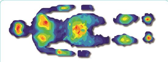
Subject shown lying on a 2-sensor configuration (model #5400N). The high spatial resolution of the sensor allows you to measure and display the high pressure areas (in red) as the subject is lying down (back of head, left scapula, right elbow, lower back, and back of heels).
